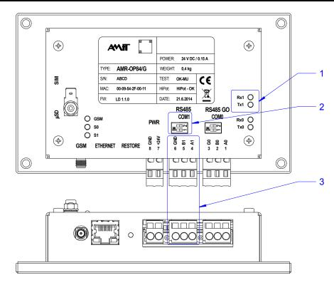
Fig. 7 - Location of RS485 line connectors
