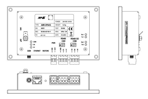
Fig. 2 - Connectors and indication elements location
