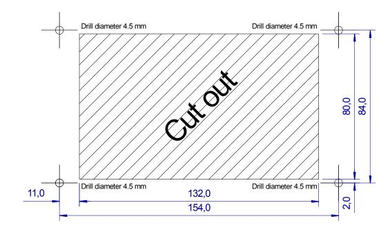
Fig. 13 - Mounting apertures
