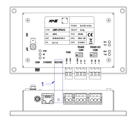
The *RESTORE* button is located on the rear side of the terminal.
