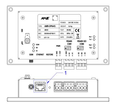
Fig. 8 - Location of Ethernet line connector
