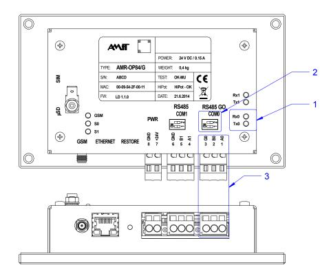
Fig. 6 - Location of galvanically separated RS485 connector
